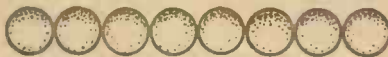
Fig. 4.—In a coil the high-frequency current all crowds towards the inside of the coil as shown here.
